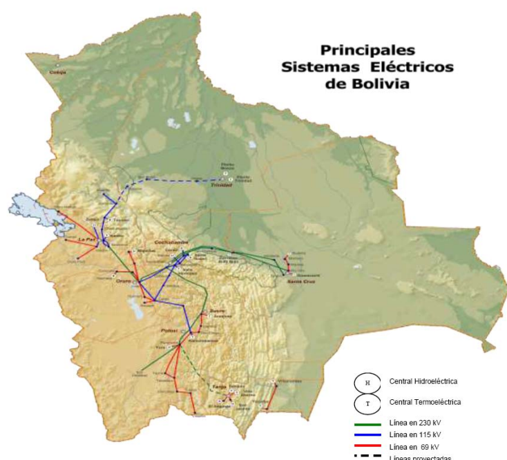
Figure 12: Main electrical systems in Bolivia
