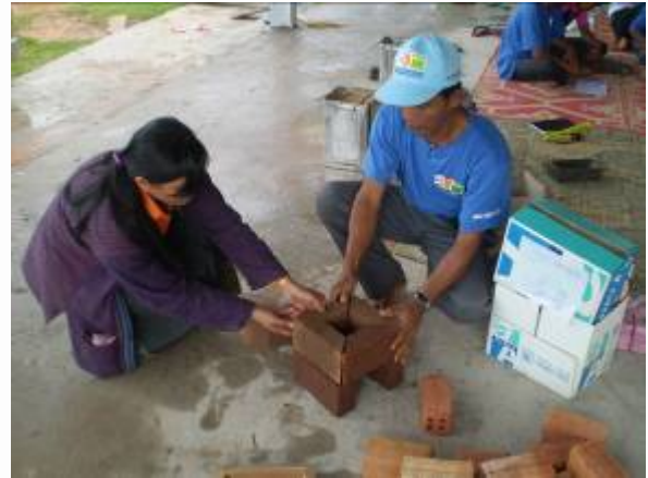
Figure 47: Level 2 trainer showing villagers (Level 3) how to assemble the rocket stove
