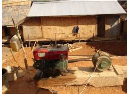
Figure 42: Rice mill engine used for sawing, lighting and entertaining
