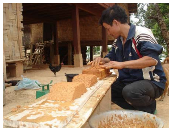
Figure 29: Course 8, Participant had really interested making of brick for constructing the rocket stove
